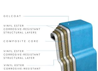
aviva Pools are built using vinyl ester resin within all layers of application providing the highest level of structural integrity and protection against osmosis (water penetration). Our degree of confidence is so high that we stand behind our products with a Lifetime Structural Warranty and a Lifetime Structural Osmosis Warranty. This is the pool that you have always dreamed of.
